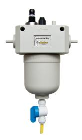
universal fm 5/3, pressure-resistant measuring cell up to 0.5 bar, for 3 electrodes (potentiostatic electrode, pH and OPR), PT1000 and flow measurement, counter electrode stainless steel (V4A)
