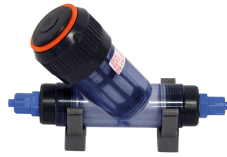
0101-120-00 Fiber filter 3/4", connection 8/6 mm with screen tube 0.5mm, hose connection 8/6 mm on both sides
